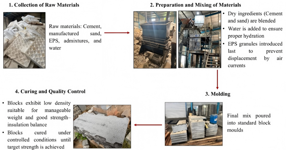
Figure 6. Manufacturing process of EPS blocks.
