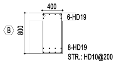
Figure 6. Beam section design.
