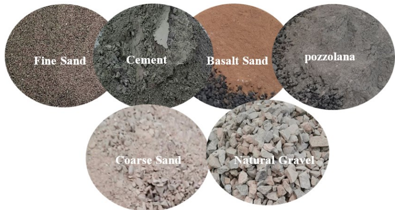
Figure 2. Materials used in concrete mixtures.
