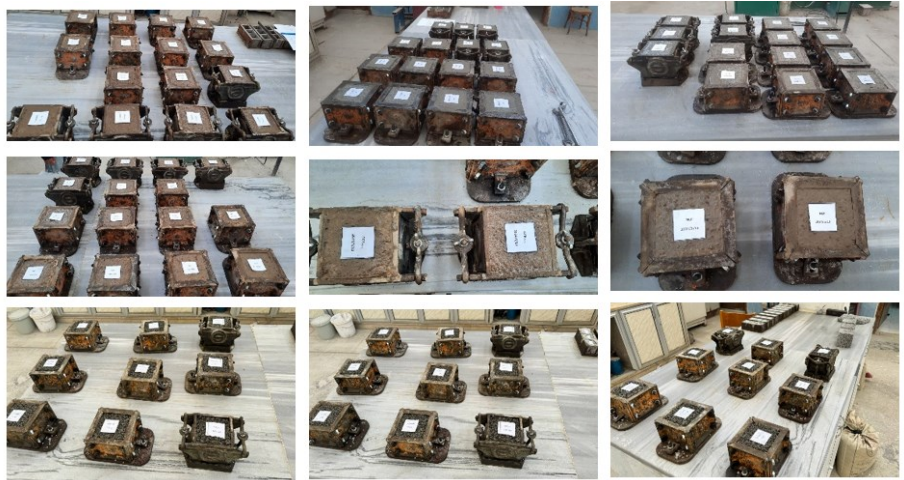
Figure 4. Casting samples in molds.
