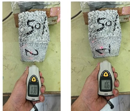
Figure 5. Measuring the difference in temperature for the first group of mixtures (GCS P50% ).
