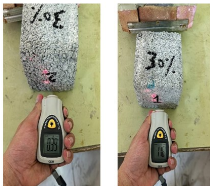
Figure 6. Measuring the difference in temperature for the first group of mixtures (GCS P30% ).
