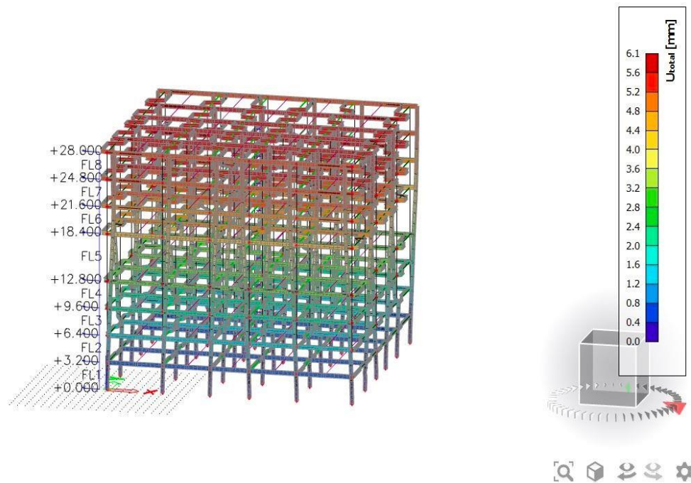
Figure 16. Displacements for case EQX (elevation irregularity).
