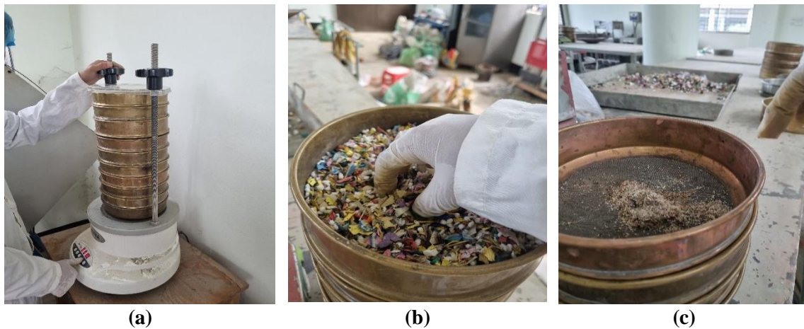
Figure 6. Sieving (a) Mechanically (b) and (c) Manually.
