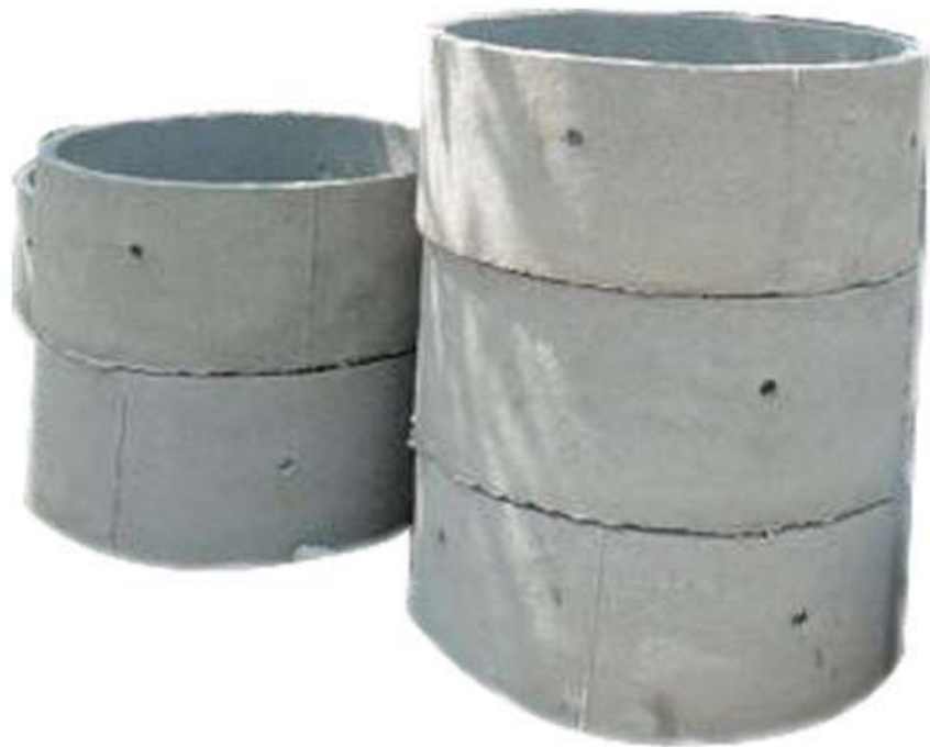
Figure 4. Typical latrine ring (diameter 30", thickness 1.5", height 12").
