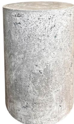
LVPW is slightly visible on the surface
