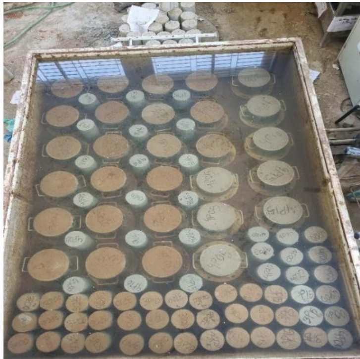
Figure 10. Concrete setup for curing.
