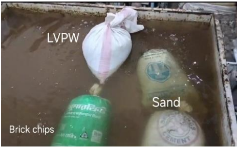
Figure 8. LVPW, sand & brick chips placed in water tank.
