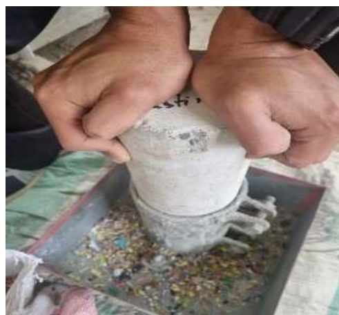
Figure 7. Compaction of LVPW.
