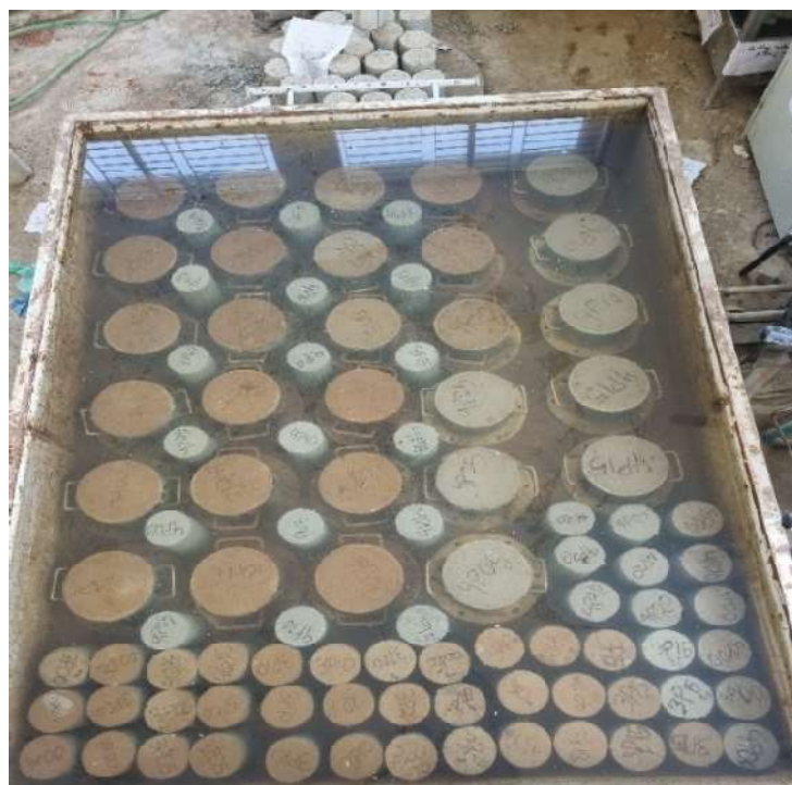
Figure 10. Concrete setup for curing.
