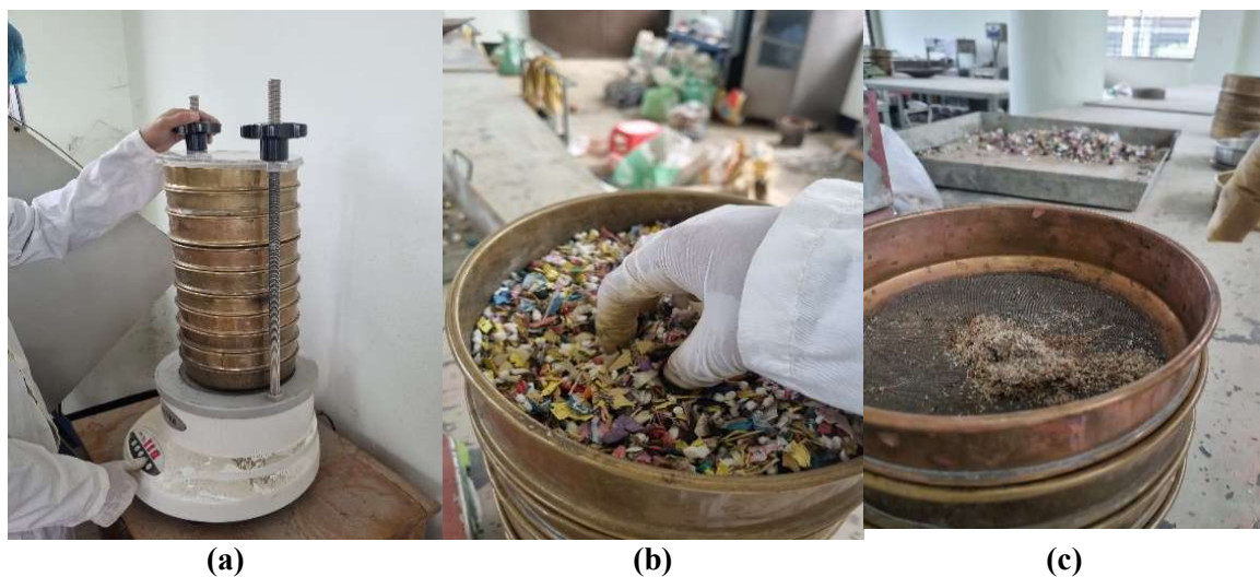
Figure 6. Sieving (a) Mechanically (b) and (c) Manually.
