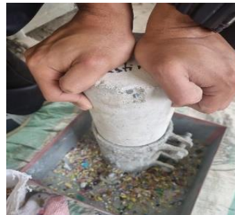
Figure 7. Compaction of LVPW.
