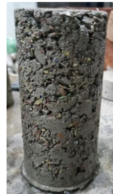
LVPW is clearly visible on surface, rough finish
