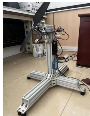
Figure 13. Motor propeller tension experimental platform.
